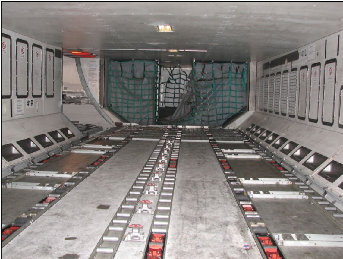
For reference only – internal detail of the A330-300 rear cargo hold. Image source: ATSB
