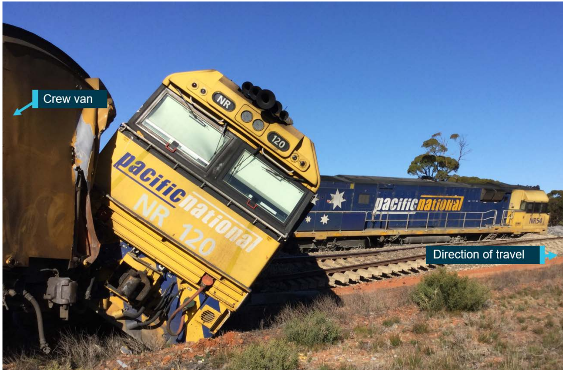
Figure 3: Derailed locomotives NR 54 (lead) and NR 120 (trailing).
