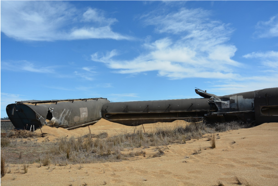
Figure 2: Derailed wagons and grain spillage
