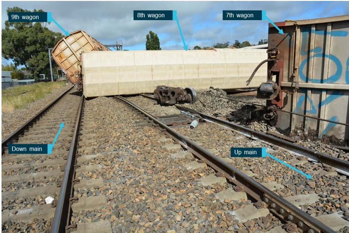
Figure 4: Derailed wagons foul of main lines
