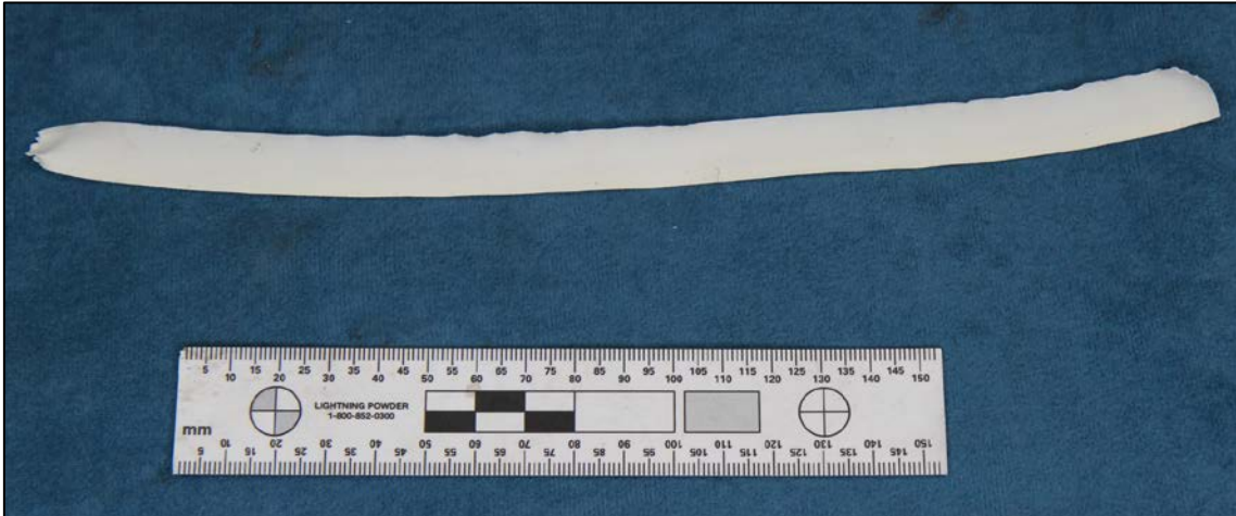
Figure 8: A section of sealant removed from a drum base.
