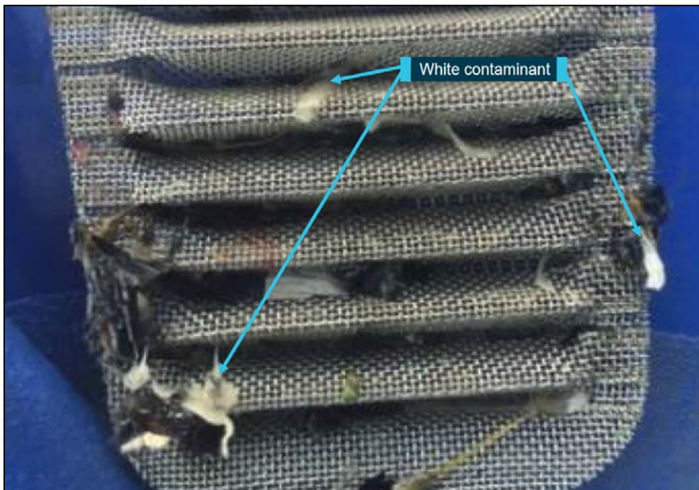
Figure 3: White contaminants in the ‘rock catcher’ – part of the fuel pump system
