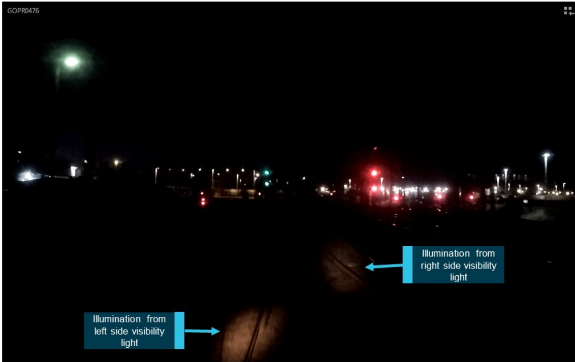
Figure 12: Similar train type showing visibility (ditch) lights illuminating track ahead
