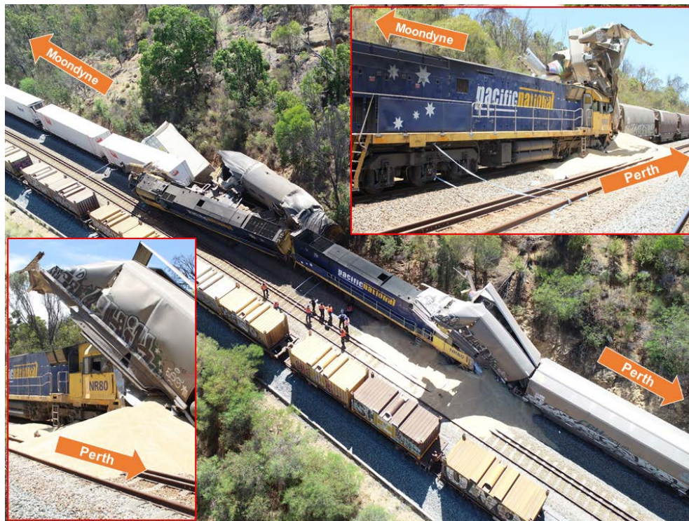
Figure 4: Accident site, lead locomotive of 7MP5 and last wagon of 2K66 post collision.
