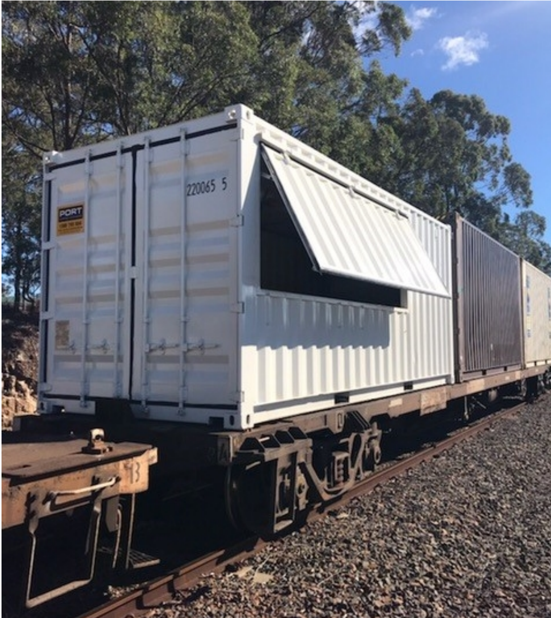
The image shows the awning open when inspected at Craven North. The container number 2200655 is also visible on the end door Source: Pacific National
