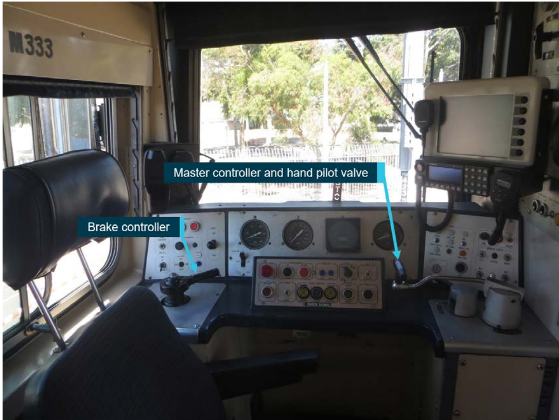
Figure 2: Comeng driver’s cab of 333M, showing location of the brake controller, and combined master controller with hand pilot valve
