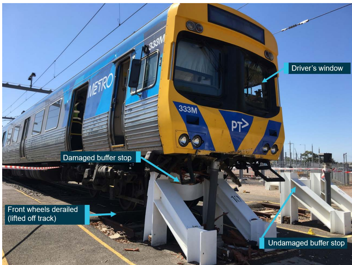
Figure 1: Front of Comeng train TD 6591, showing collision with buffer stop and derailment
