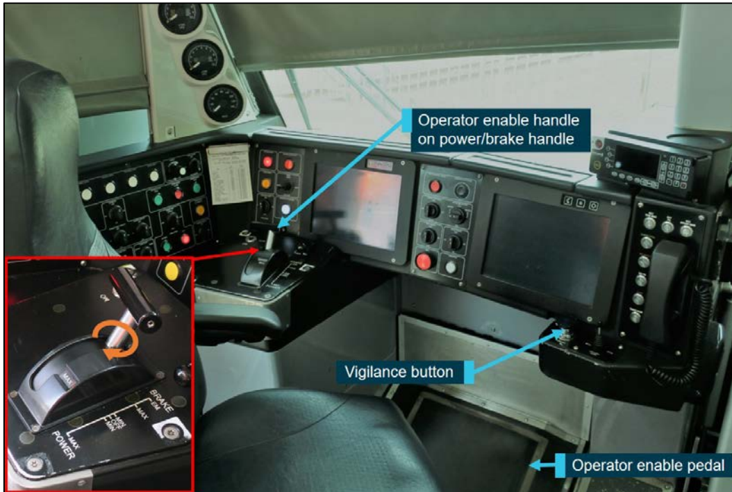
This figure shows the location of the driver safety systems on A42. The insert shows the power / brake handle and the twist grip which acts as part of the operator enable system. Source: ATSB
