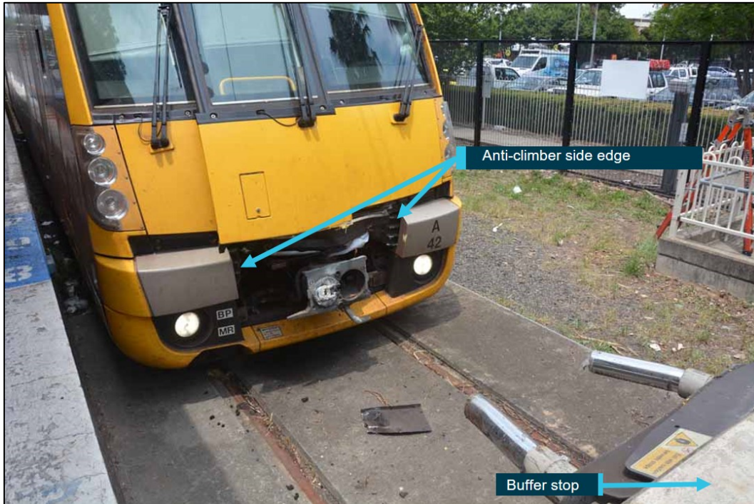
This figure shows position of the anti-climbers on the leading car of A42 and the edge which contacted the buffer tube flange. Source: ATSB
