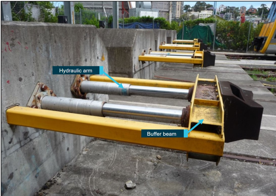
This figure shows an energy-absorbing hydraulic buffer stop. It has hydraulic rams, a buffer beam and a coupler-compatible arrangement at the front. Source: TfNSW with annotations by ATSB
