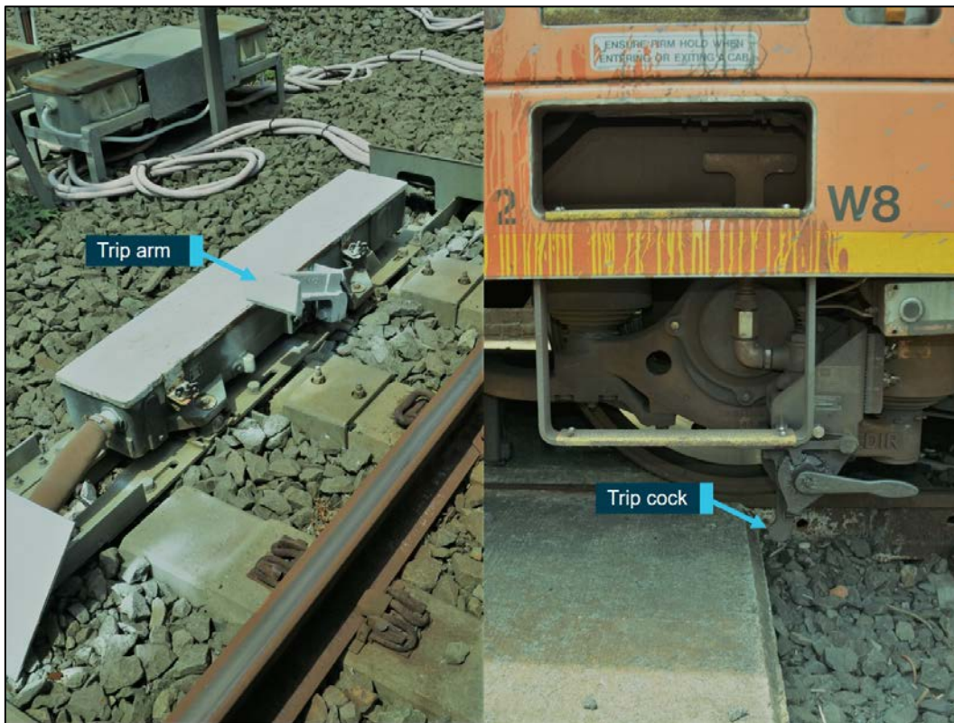
This figure shows the trip arm next to signal RD5 at Richmond (left) and the trip cock on A42 (right). Source: ATSB
