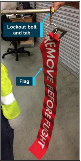
Figure 2: Maintenance lockout bolt
