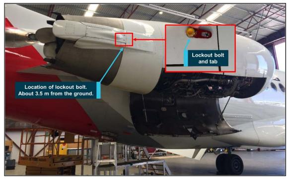
Figure 3: Photograph of right engine with an exemplar in-service thrust reverser lockout bolt
