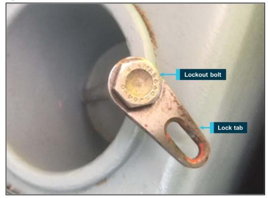
Figure 1: In-service thrust reverser lockout bolt and lock tab
