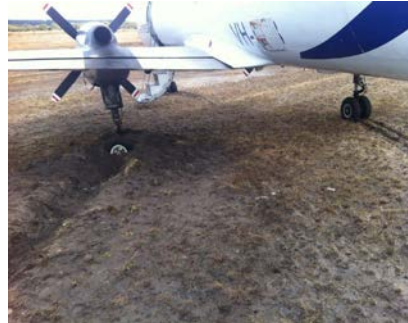
UUB after veering off runway
