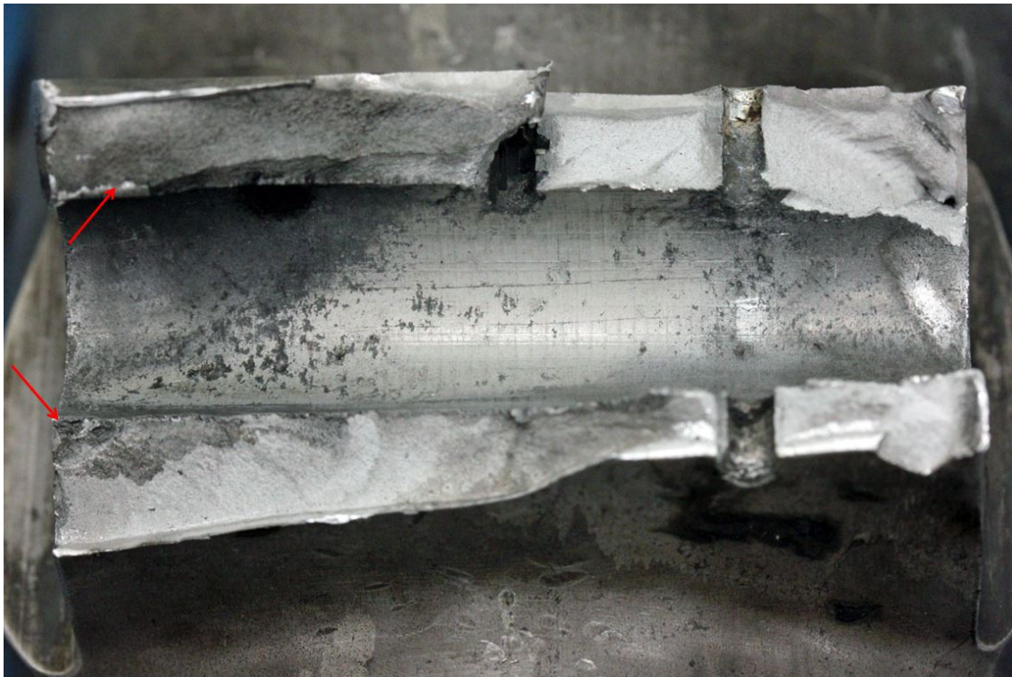
Figure 5: Yoke lug exhibiting corrosion pitting, wear in the bore and fatigue crack progression on the fracture surfaces (main crack origins arrowed)
