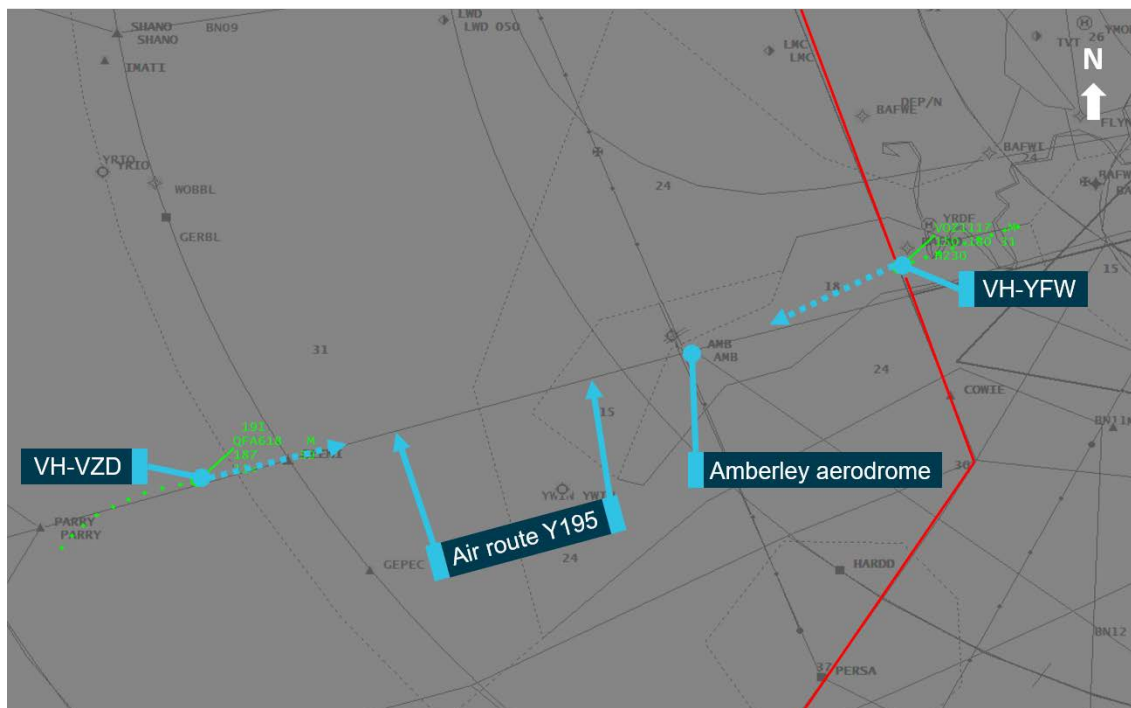
Figure 1: Position and direction of the two aircraft when VH-YFW entered Amberley airspace at 1411:44. The red line indicates the boundary between Brisbane airspace (right) and Amberley (left) airspace. Air route Y195 was assigned to VH-VZD.
