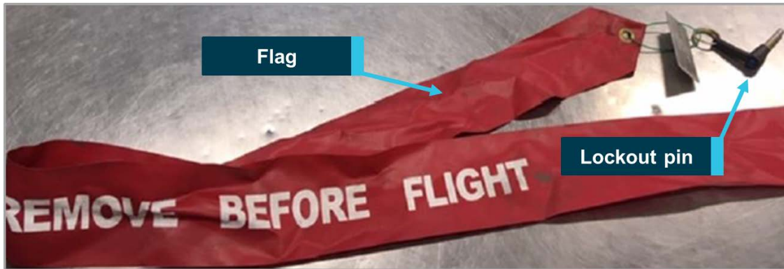
Figure 1: Photograph of a thrust reverser lockout pin and warning flag (non-reflective)
