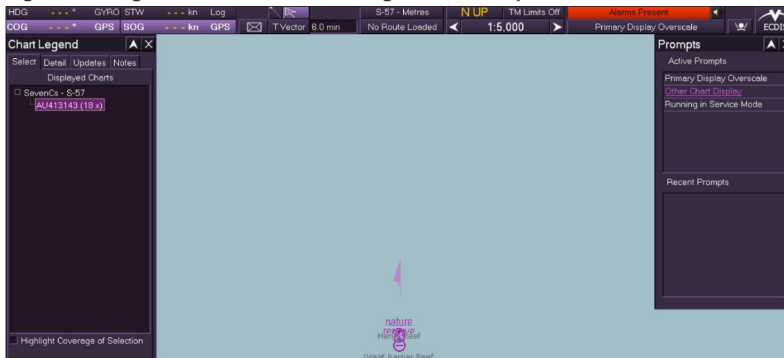
Image of a VisionMaster FT ECDIS display showing ENC AU413143 at a scale of 1:5,000 and displaying no overscale pattern. Source: Northrop Grumman Sperry Marine, modified by the ATSB
