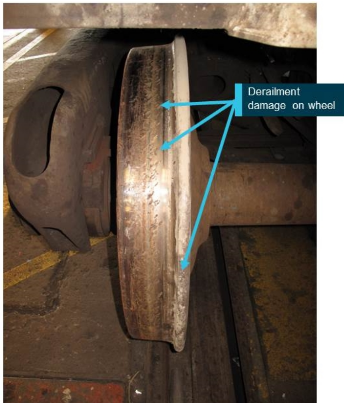
Figure 7: Wheel damage (all four wheels displayed similar damage)
