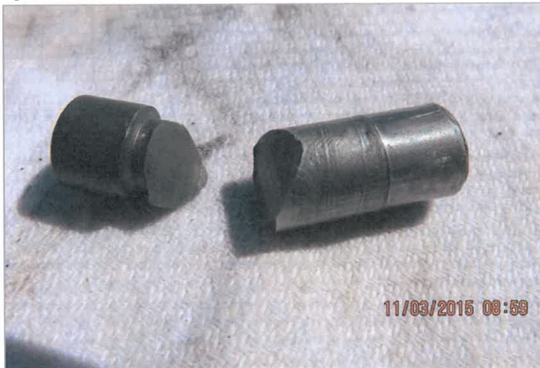
Figure 1: Failed nose landing gear downlock pin
