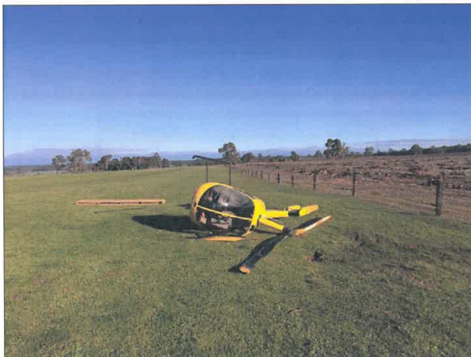
Figure 2: VH-RBT at rest on the left side. Note the broken tail boom and rotor blades
