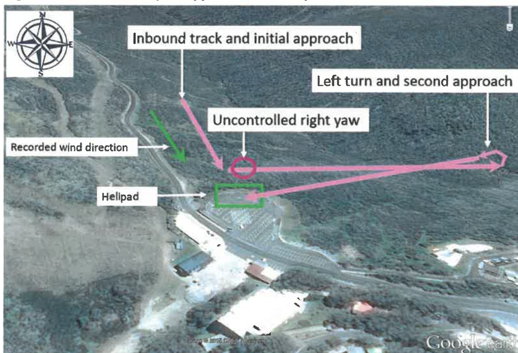
Figure 1: Falls Creek helipad, approximate helicopter track and wind direction
