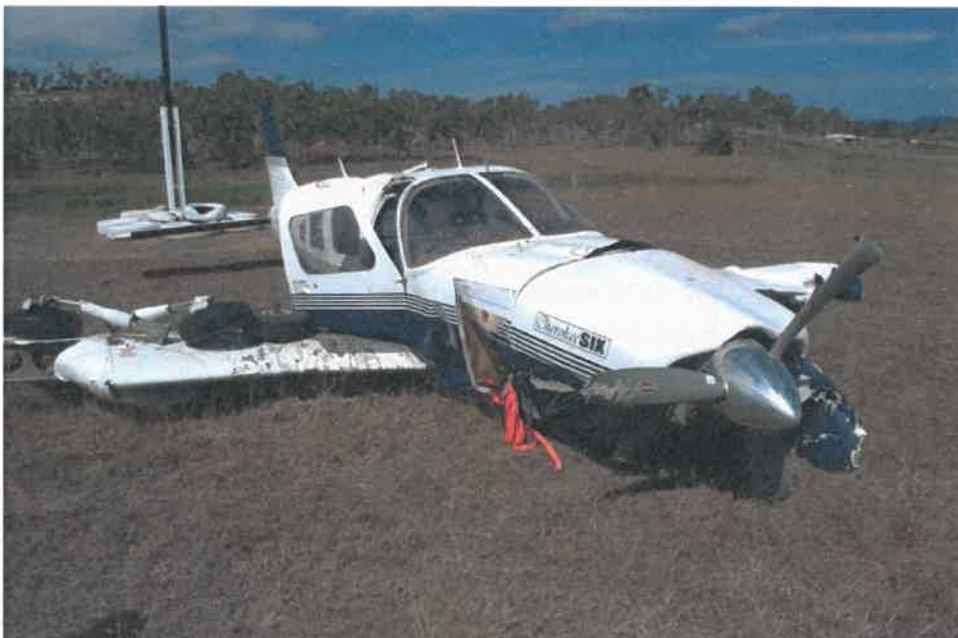
Figure 6: VH-BDG after retrieval from the lake. Passenger 2 (below) reported that the left wing crumpled during the 'cartwheeling' toward the lake. Note: Significant damage occurred during the retrieval process
