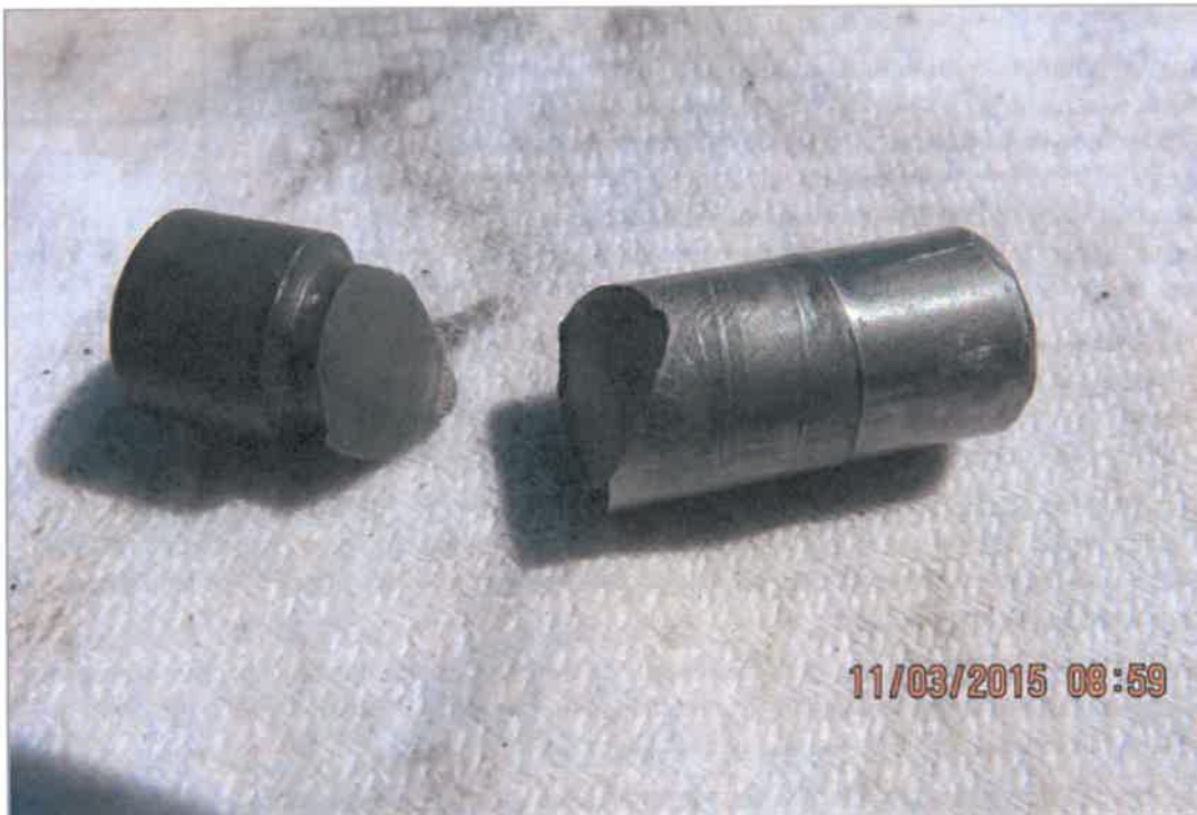
Figure 1: Failed nose landing gear downlock pin
