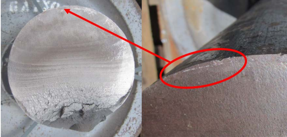
Figure 7: White paint on fracture surface near origin
