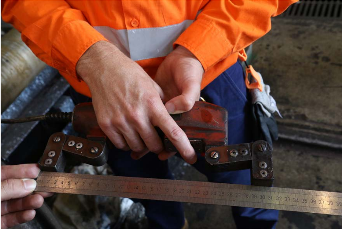
The measured width of the AC yoke on the day of the site visit. Source: ATSB
