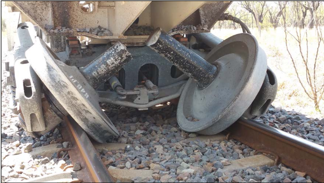
Figure 2: Failed axle in-situ from train 9T90
