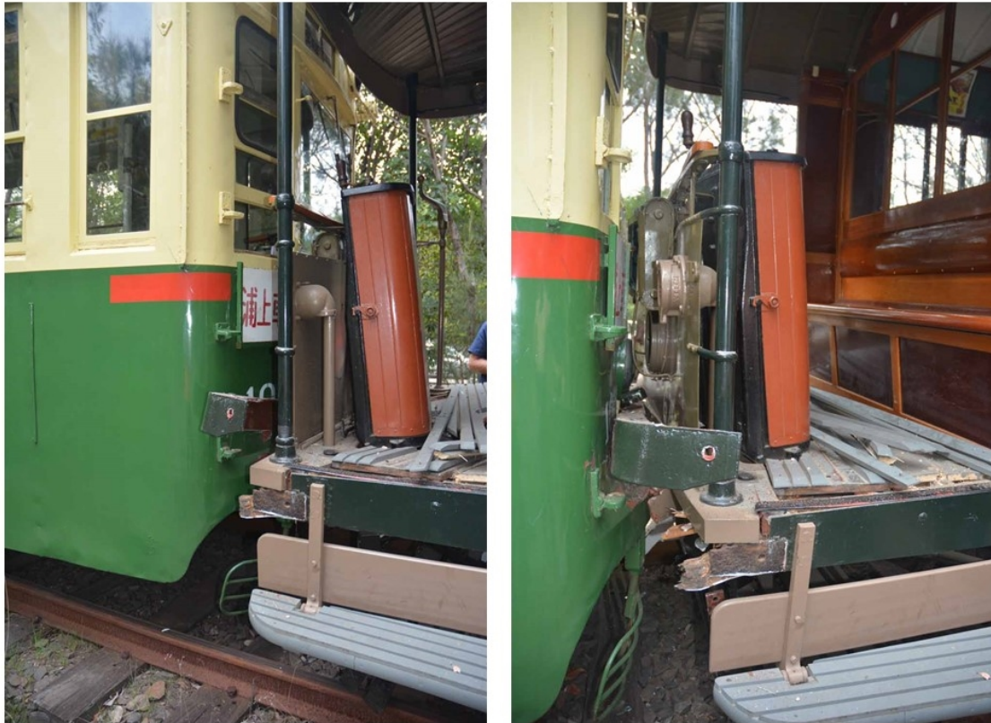
Figure 6: Damage to the 675 'J' class tram
