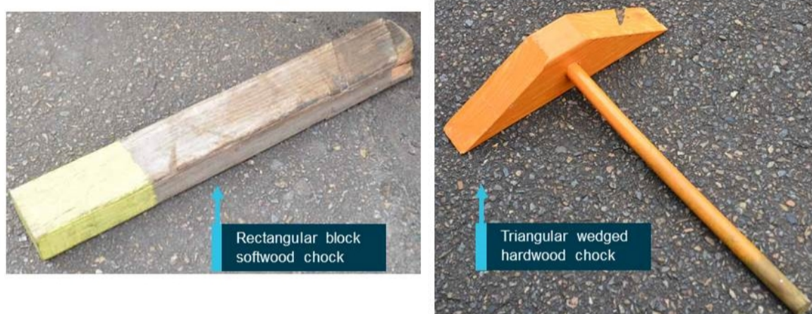
Figure 8: Comparison of the old and new type chock
