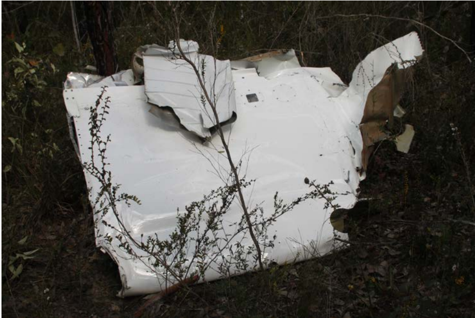
Figure 6: Right wing inboard section in as found position (zone C)
