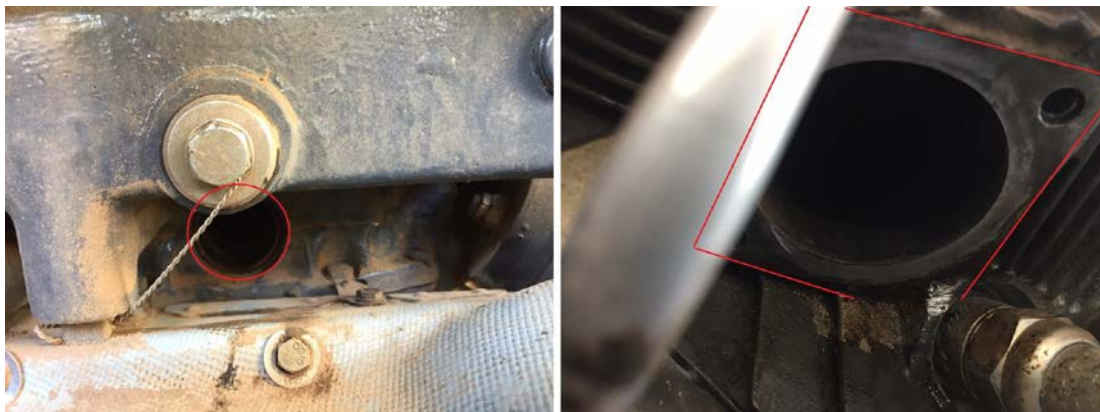
Figure 3: Lower (left image) and upper (right image) air intake pipe attachments points highlighted in red. Air intake pipe, bolts and flange are missing.
