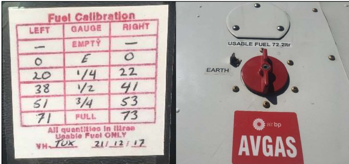
Figure 2: Fuel placard and label installed on VH-TUX
