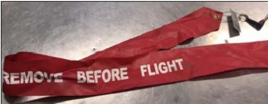
Figure 2: Lockout pin with warning flag
