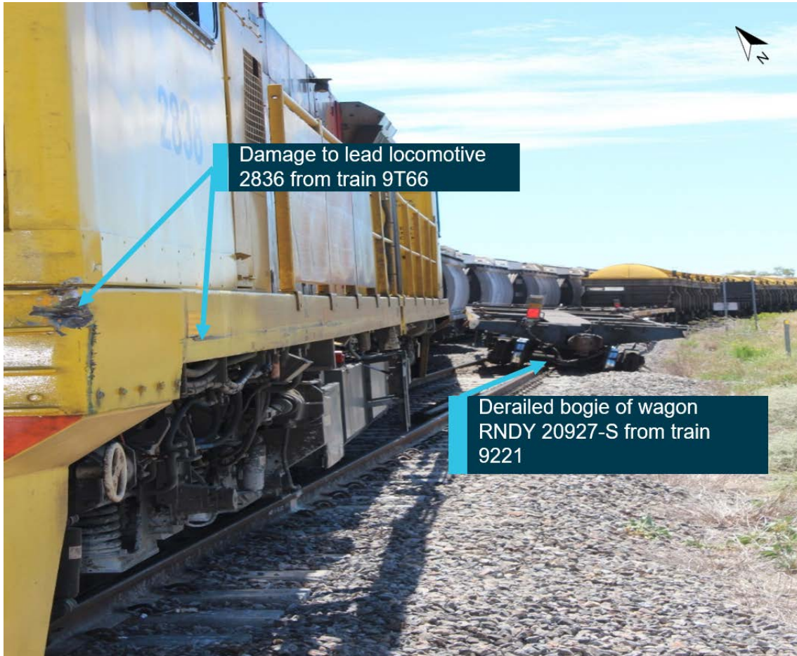
Figure 2: Damage to locomotive 2838 and wagon RNDY 20927-S
