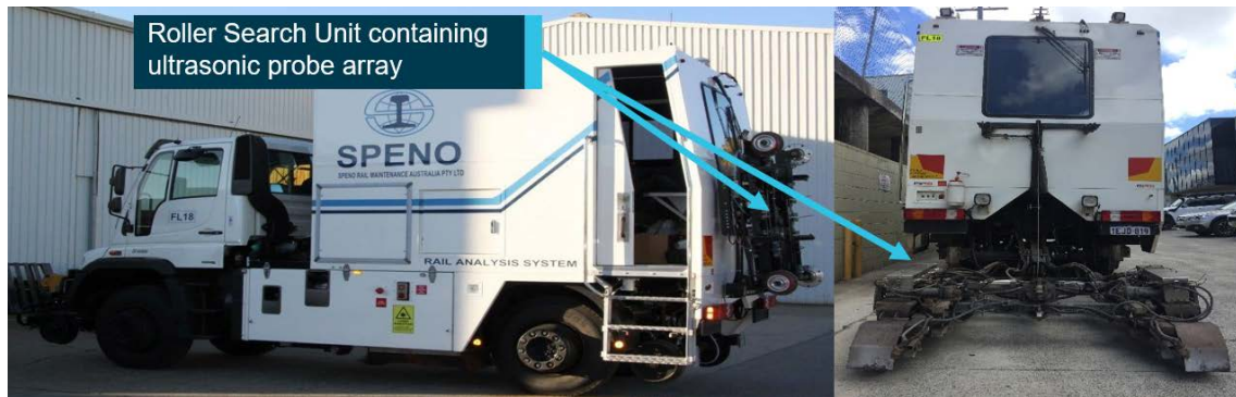
Figure 5: FL-18 (RFAS-2100) rail analysis system (main test vehicle)
