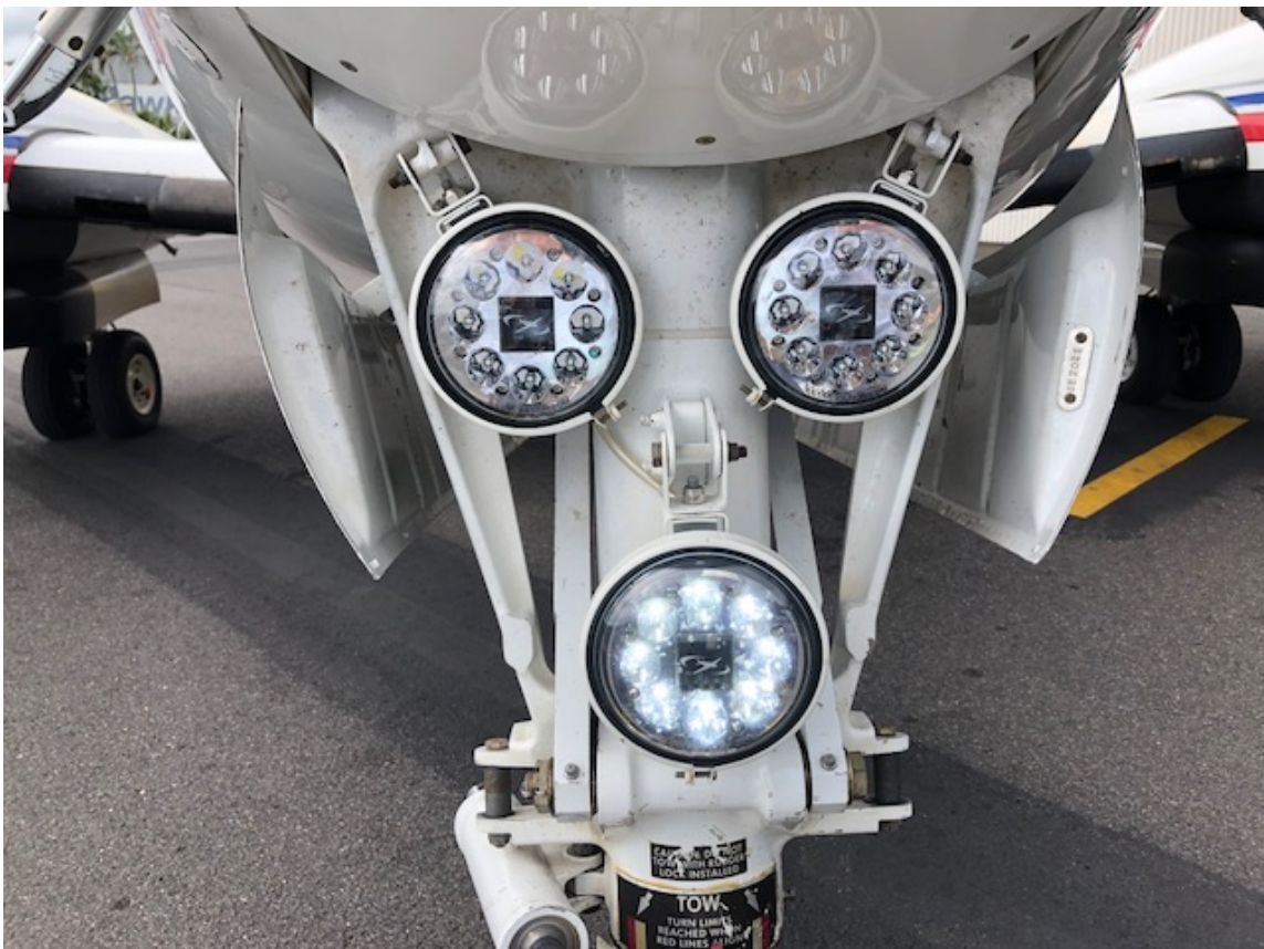
The nose gear of a RFDS Beech B200 fitted with LED lights for landing (outer) and taxi (centre). Source: Royal Flying Doctors Service
