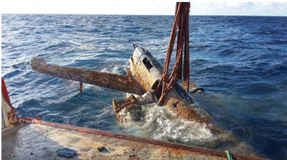
Figure 1: The tail section of VH-NGA being recovered by Pacific Marine Group for the ATSB.
