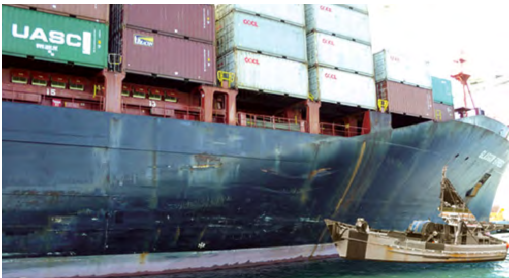
Figure 12: Composite representative image showing the scale and approximate point of collision
