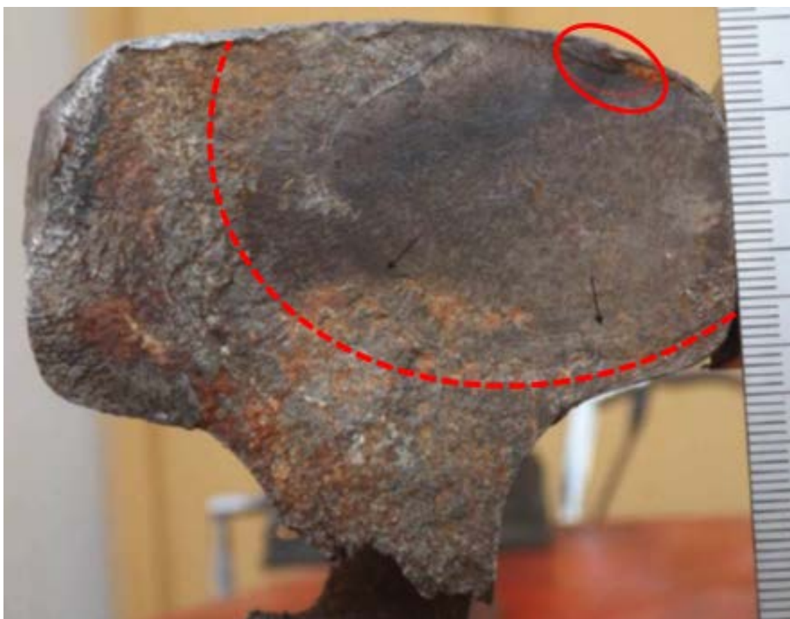
Figure 12: Large fatigue crack in rail section
