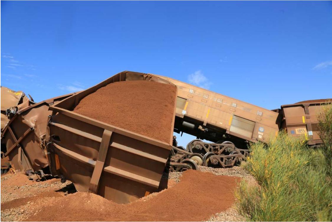
Figure 3: Derailed, loaded iron ore cars located in the rear portion of train M03544
