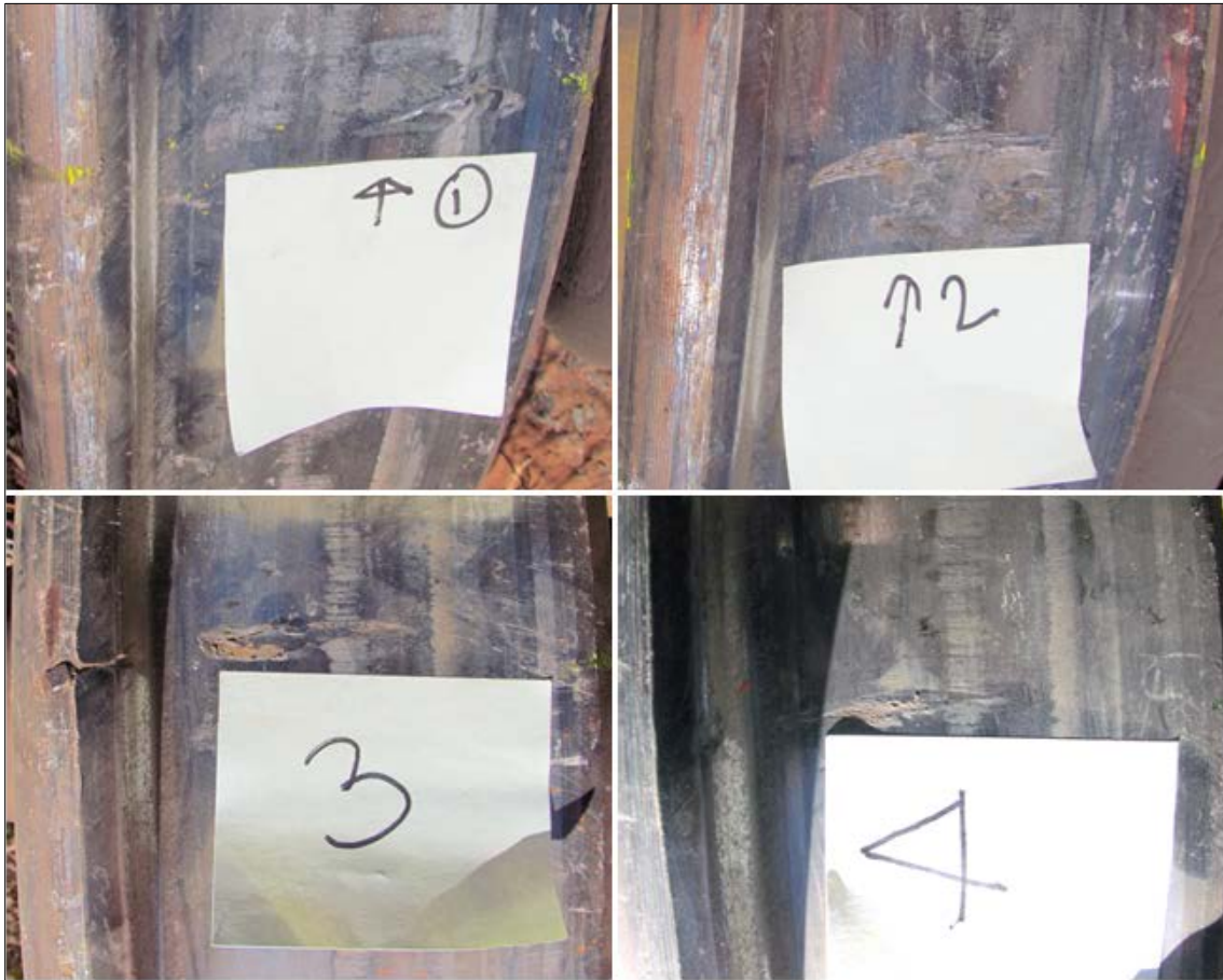
Numbered 1 – 4, corresponding rail impact bruises on the wheel tread surface (Figure 6) on ore car 8934 - wheelset #2L. All impact marks are transverse, angled about 90° across the tread surface. - Source: BHP Billiton.
