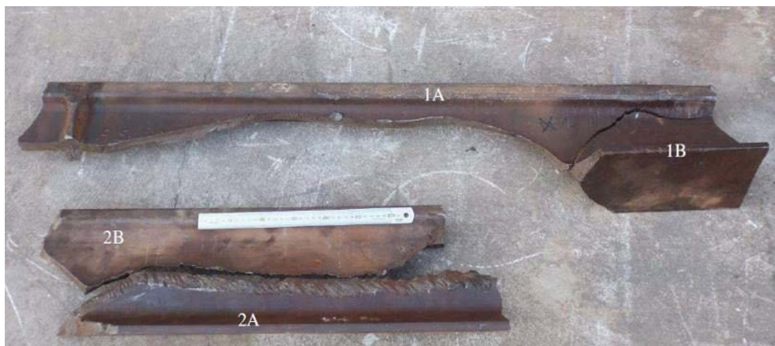
Figure 11: Broken rail with fatigue cracks
