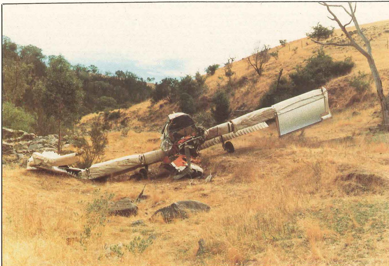
The aircraft was returning to the operations base after spreading superphosphate at a nearby property. While flying along the river it hit a power line which spanned the gorge, 300 feet above the river. The aircraft crashed on to the river bank and the pilot was killed.
