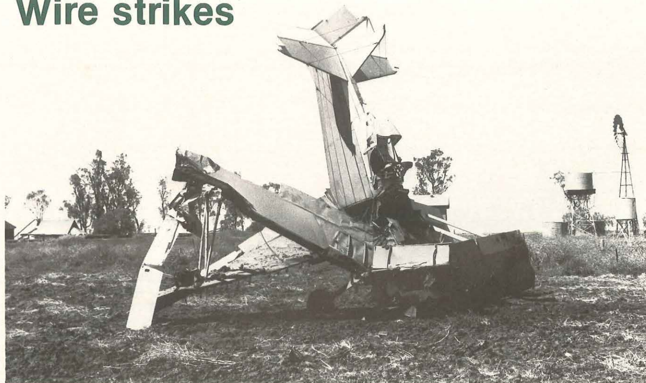
'The cause of the accident was that the pilot did not maintain the high degree of vigilance which is necessary when conducting agricultural spraying operations'.
