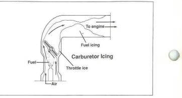
It is possible that all three types of icing will be encountered at the same time, but that arising from fuel evaporation is the most likely except in extremely cold conditions.
