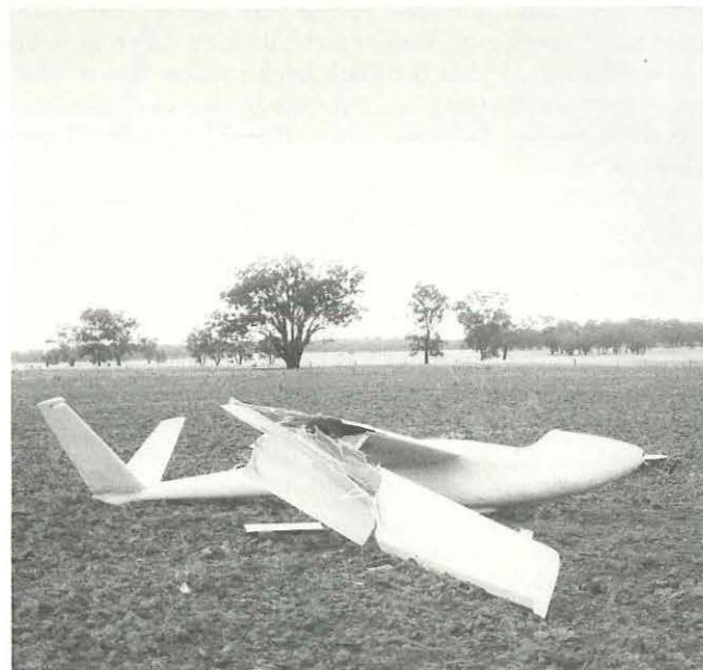
The wrecked Pilatus (left) and Salto (right) as they came to rest in open country after the collision. Note the entire tail section of the Pilatus has been torn away.
