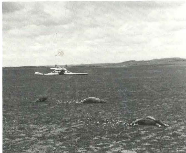
View of paddock from which Cessna was operating, looking in direction of take-off. Three of the four sheep the aircraft struck, and the dislodged nose wheel, can be seen in the picture.
