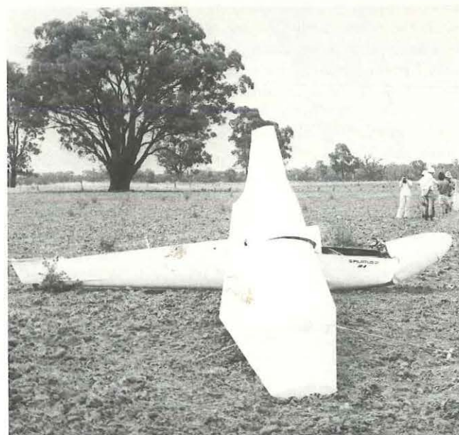
The wrecked Pilatus (left) and Salto (right) as they came to rest in open country after the collision. Note the entire tail section of the Pilatus has been torn away.
