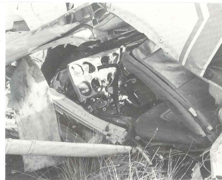
The degree of compression of the nose and cabin area is evident in both of these photographs.
