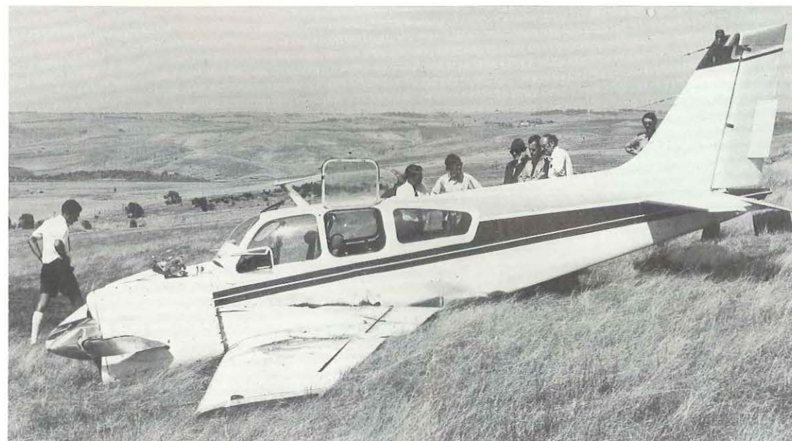
Left: General view of aircraft as found. The chart obscuring the port windscreen panel can be seen still in position. Note the surprisingly intact appearance of the aircraft for this type of accident.
