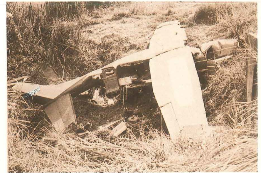
Above: The collapsed and distorted airframe as it came to rest against the creek bank.
