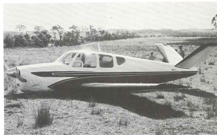
Opposite Page:— Above: The aircraft as it came to rest in the paddock, looking in the landing direction. The touchdown marks are visible in the foreground.
