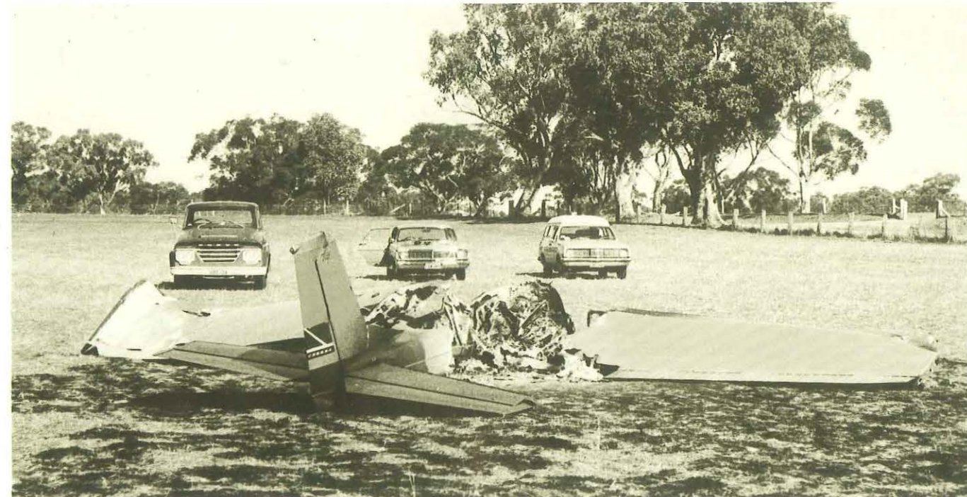
The gutted wreckage of the Cessna 150. It is possible that the power line and rising terrain in the background affected the pilot's judgement.
