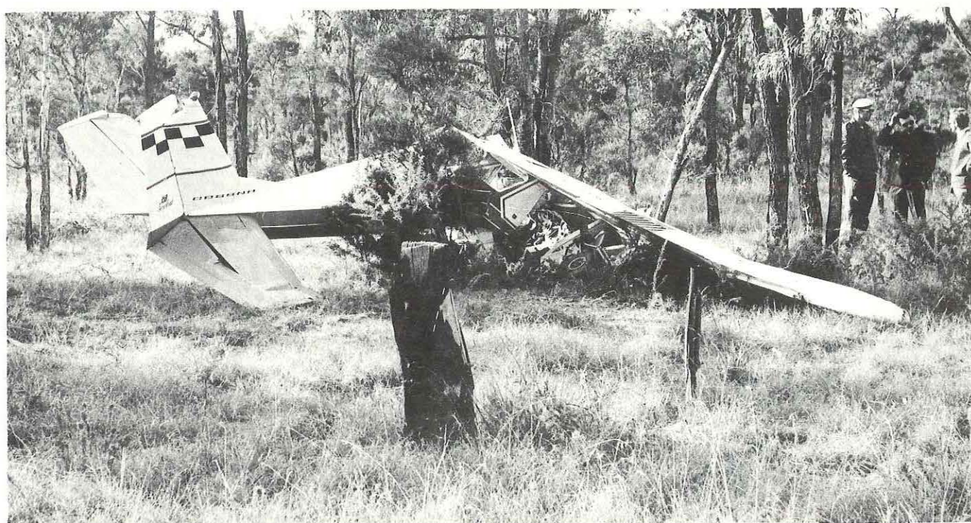
The wreckage as it came to rest. The steep nose-down attitude on impact is clearly evident.
