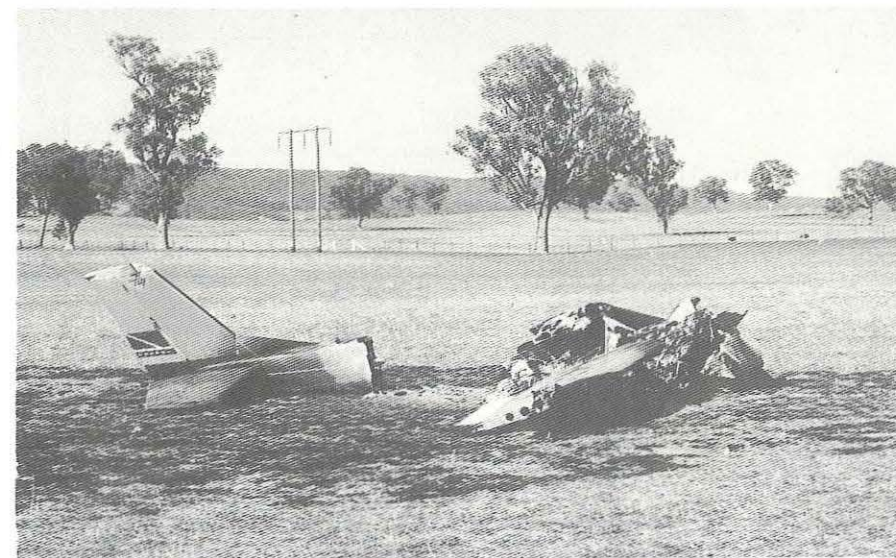
The gutted wreckage of the Cessna 150. It is possible that the power line and rising terrain in the background affected the pilot's judgement.
