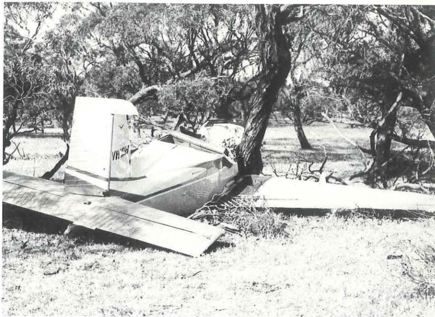
Above: The final impact site. Note the tree which has penetrated the cockpit area on the starboard side.
