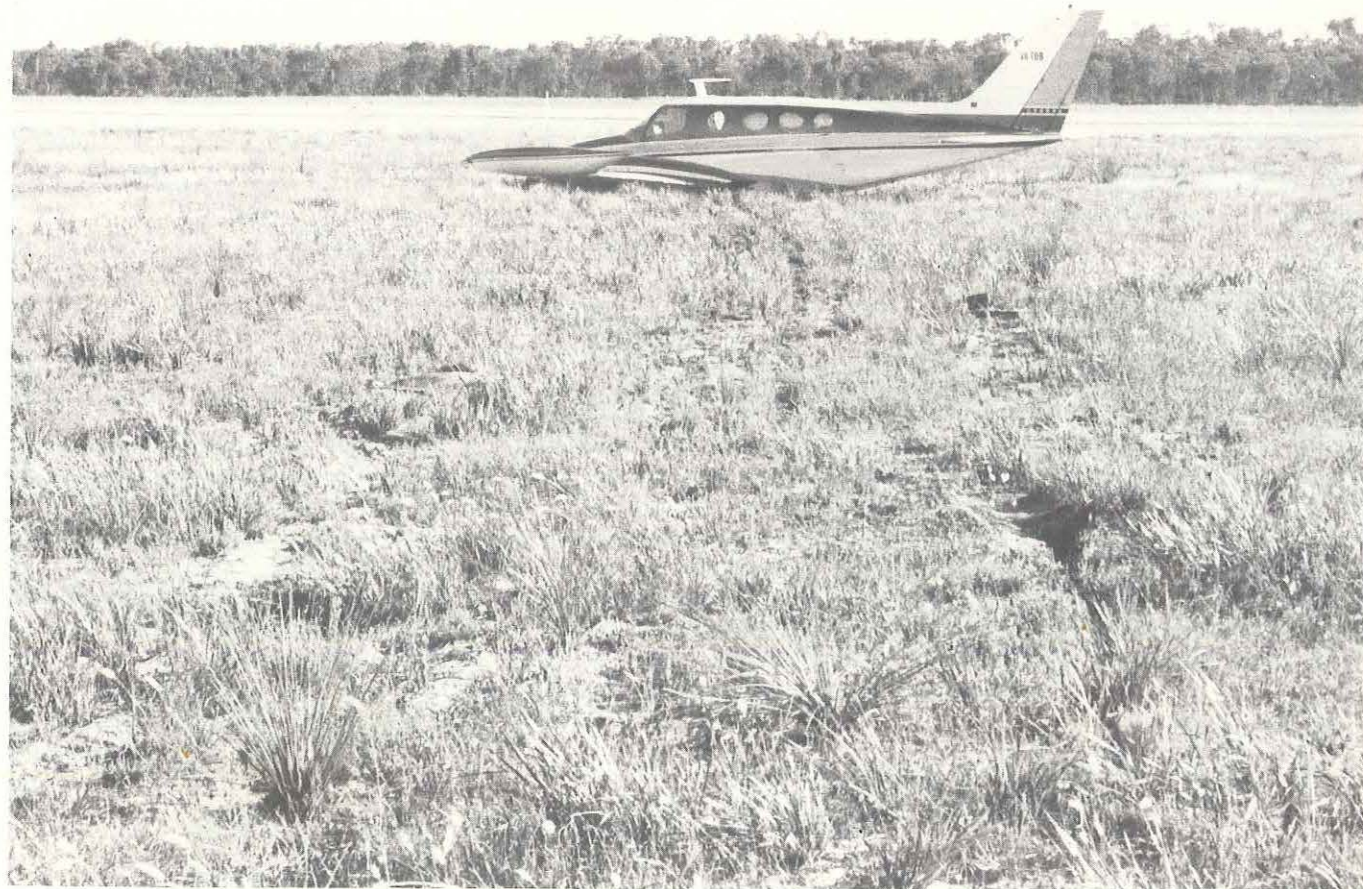
The Cessna 411 aircraft as it came to rest looking in the direction of flight. Impact and slide marks are clearly discernible in the foreground.
