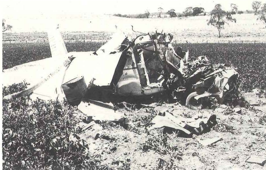
Above and Below: The remains of the Cessna 180 as it came to rest. The upper picture was taken looking in the direction of impact and portion of the wreckage trail can be seen in the foreground. Note the almost complete destruction of the forward section of the fuselage.
