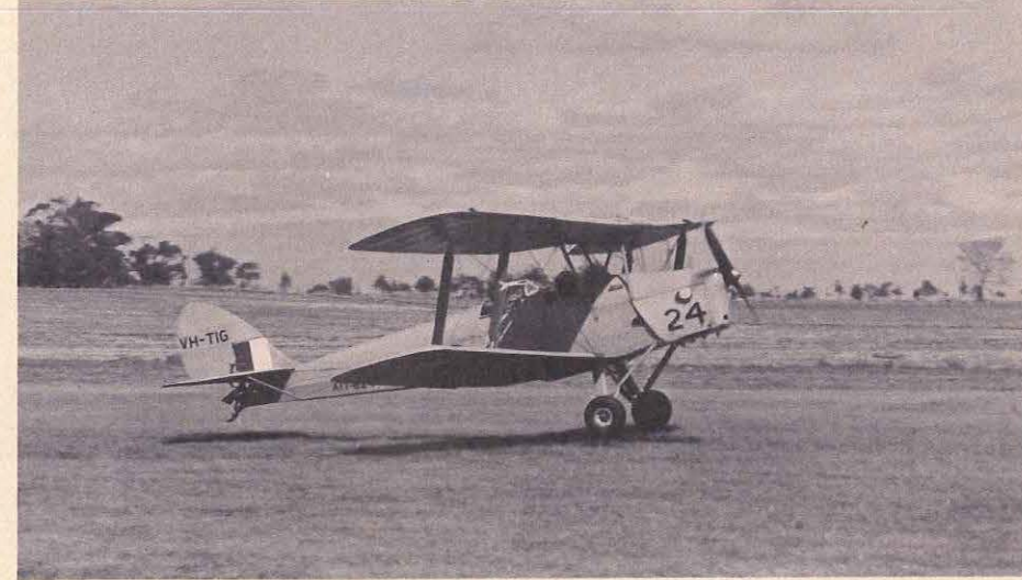
Landing: All set for a three-point! "The drag of the tail skid tends to restrain any tendency for the aeroplane to swing."
