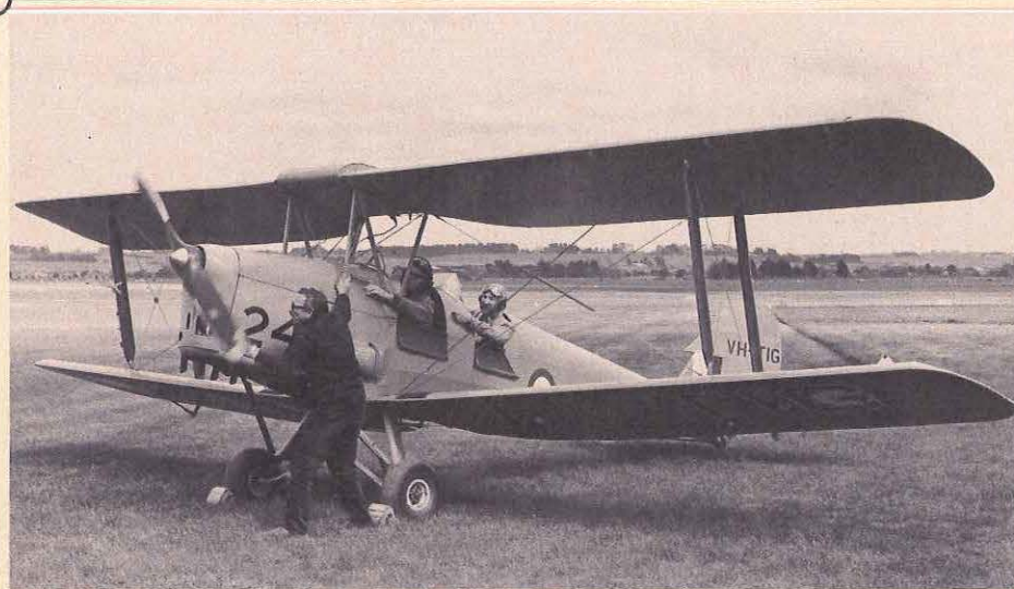
Above: "Hand swinging from 'behind' gives immediate access to the front cockpit switches."
