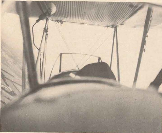
"Any lack of instrumentation is more than compensated for by the excellent attitude cues provided by the centre-section bracing wires." Left: A medium turn. Right: A steep turn.
