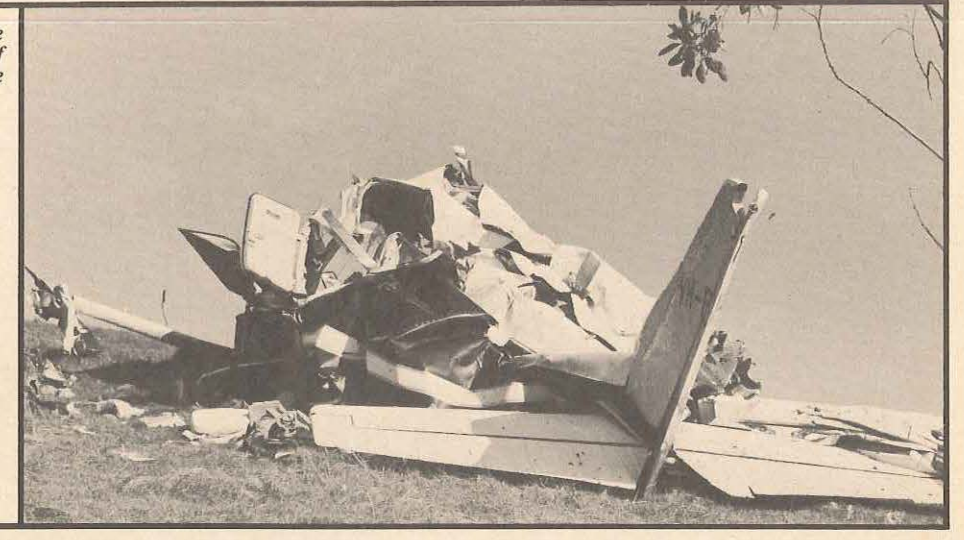
The almost complete destruction of the forward section of the fuselage is indicative of the force with which the aircraft struck the ground.
