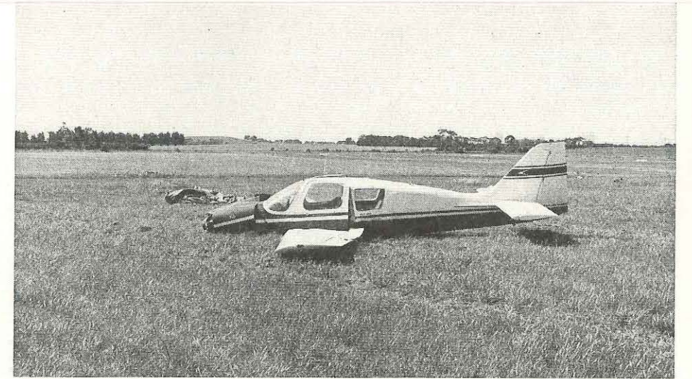
Right: Though at first glance the Beagle Pup appears relatively intact, the high vertical deceleration forces of the impact are evident on closer inspection.
