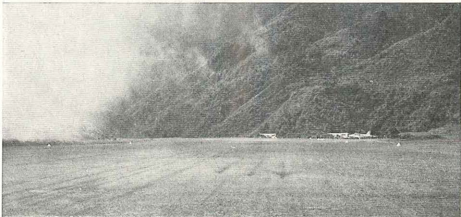
View looking in landing direction showing marks of heavy braking. The damaged aircraft can be seen at the end of the strip. Note the cloud rolling in from the left side of the strip.
