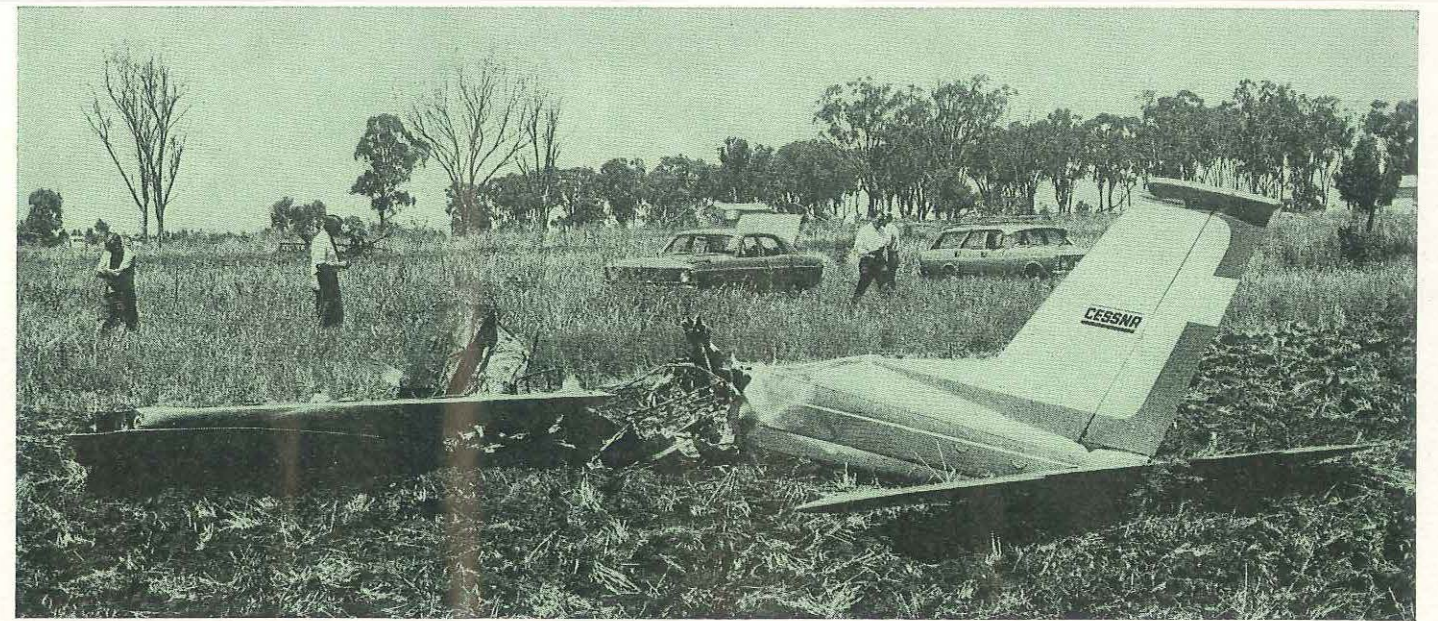
View of wreckage looking in direction of impact. The flaps are almost fully retracted.
