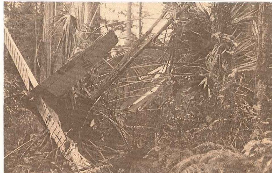
Rear view of the extensively damaged aircraft. The heavy timber and the dense undergrowth are clearly evident in this picture.
