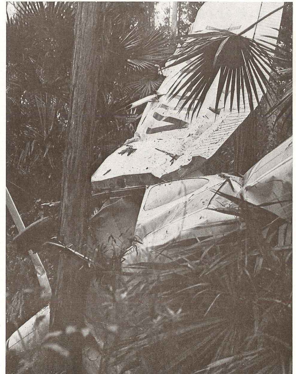
Close-up of aircraft, showing cabin area and dislodged port wing lying across the top of the fuselage. Fuel from the port tank drenched the occupants before they could extricate themselves from the wreckage.
