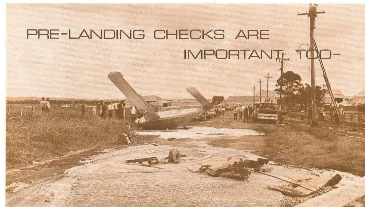
Fuel starvation on final approach can be even more embarrassing than at cruising height!
