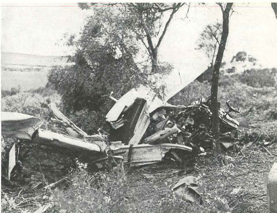
The main wreckage lying in the group of trees which finally brought it to rest. In this picture, the starboard wing has been pulled clear to gain access to the cabin area.
