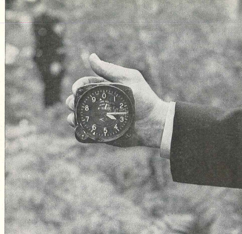
The aircraft's altimeter as recovered from the wreckage showing the reading at time of impact. The area QNH altimeter setting current at the night of the accident was correctly set on the instrument's pressure sub-scale.
