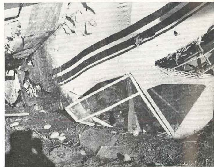
A close up of the cockpit showing the degree of impact and fire damage.
