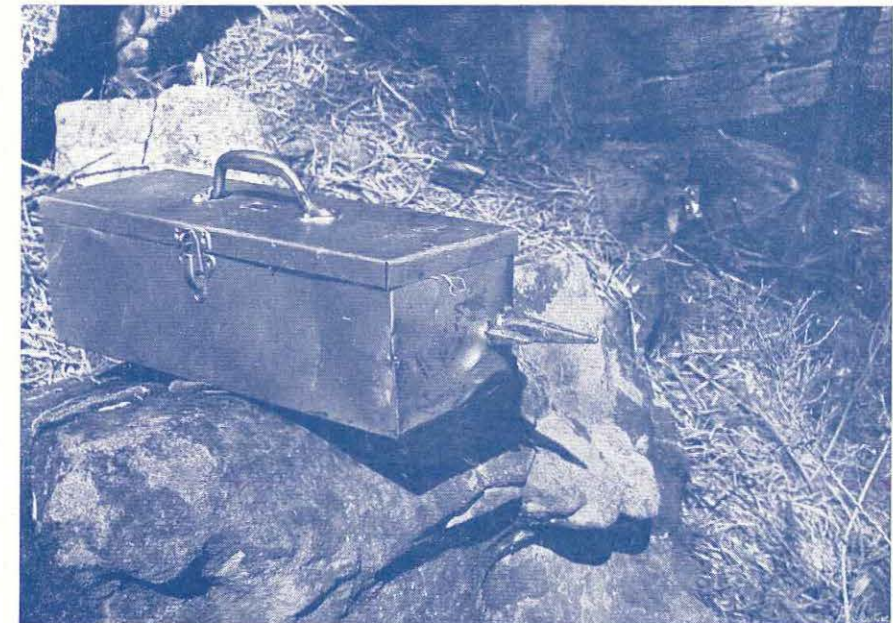
Some idea of the deceleration forces during the impact is conveyed by the damage sustained by this tool box. Two tie-down pegs contained in the box have penetrated its steel sides to a depth of three inches.
