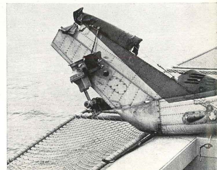
Below: The failed tail fin, showing the tail rotor hub and gear box torn away and retained only by the control cables.
