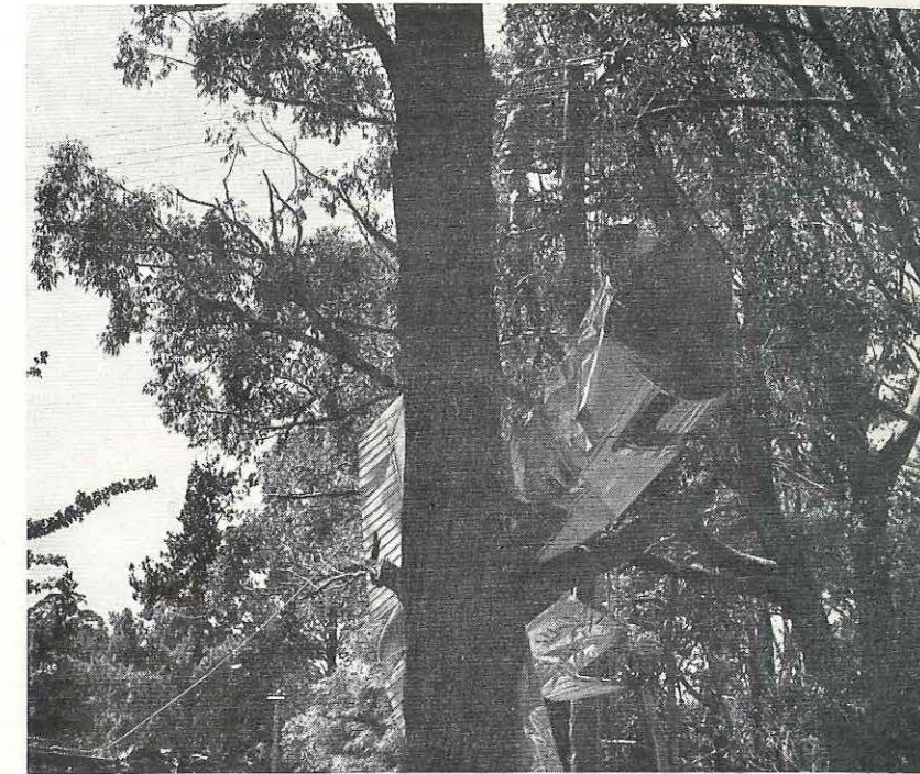
Above and Below: The disintegrated remains of the Cessna 182 after it had crashed through the trees, struck a power line, and fallen to the ground. Note the rear fuselage caught in a fork of the large tree in the picture above.
