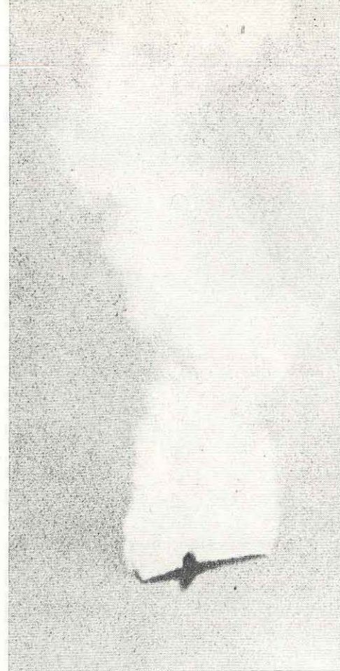
The fuselage and main portion of the wing, descending in a flat spin. The tail section is missing and portion of the starboard wing is just breaking away.
