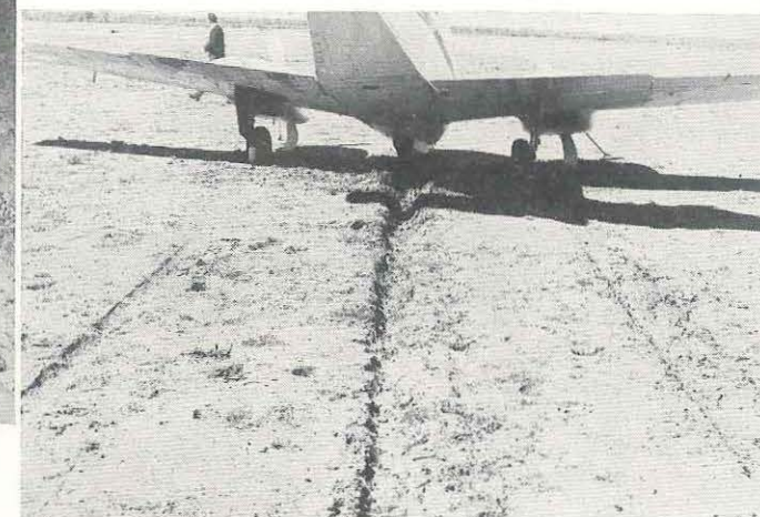
After making a normal landing on an apparently serviceable outback aerodrome, the nose-wheel of this light twin broke through the surface crust and sank 11 inches into the mud beneath. The resulting drag collapsed the nose-wheel strut. Heavy rain had fallen during the three weeks preceding the accident.
