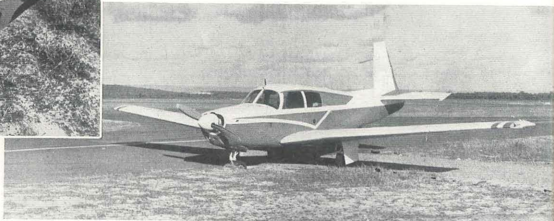
The result of manoeuvring outside the boundaries of prepared movement areas. Note the damage to the propeller.
