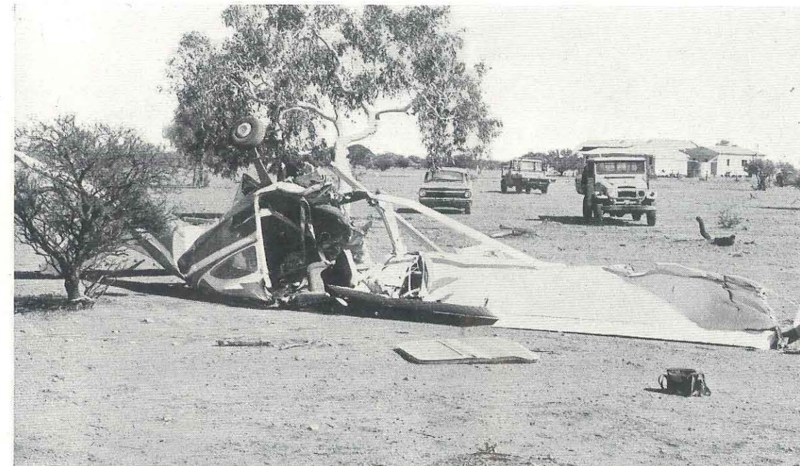
The wreckage of the aircraft as it came to rest, looking in the direction of impact. The shearers' quarters, near which some of the eye witnesses were standing, can be seen in the background.
