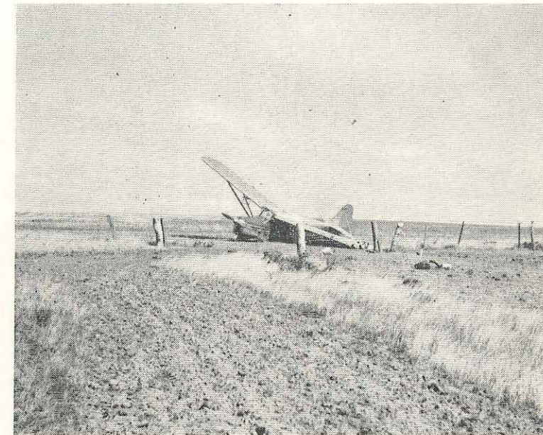
Carburettor icing forced this Auster down only a few minutes after taking off. The aircraft struck a fence during the landing.
