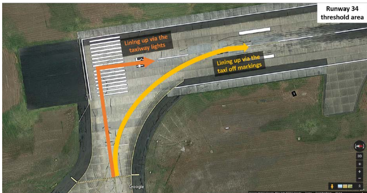
Figure 4: Threshold of runway 34 at Melbourne Airport, showing the curved line-up track in yellow, and the track in orange that follows the taxiway lighting
