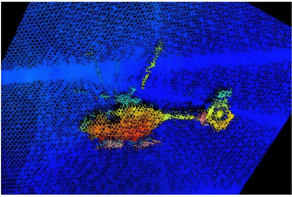
Figure 5: Sonar image of helicopter resting on the seabed, on its right side
