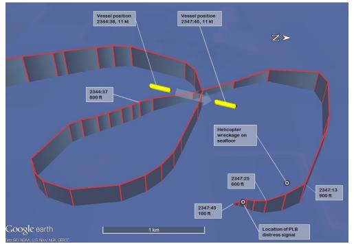
Figure 3: Ground track of the helicopter in vicinity of the departing bulk carrier
