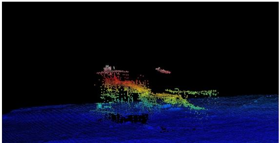
Figure 4: Sonar image of helicopter resting on the seabed, on its right side
