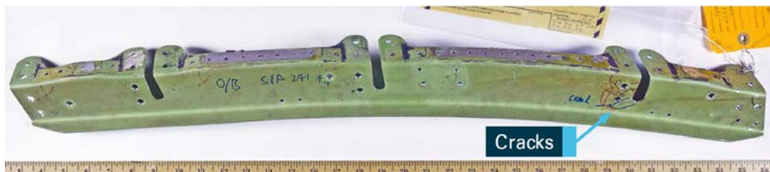
Figure 4: The strut rib from Figure 3 after removal from the pylon
