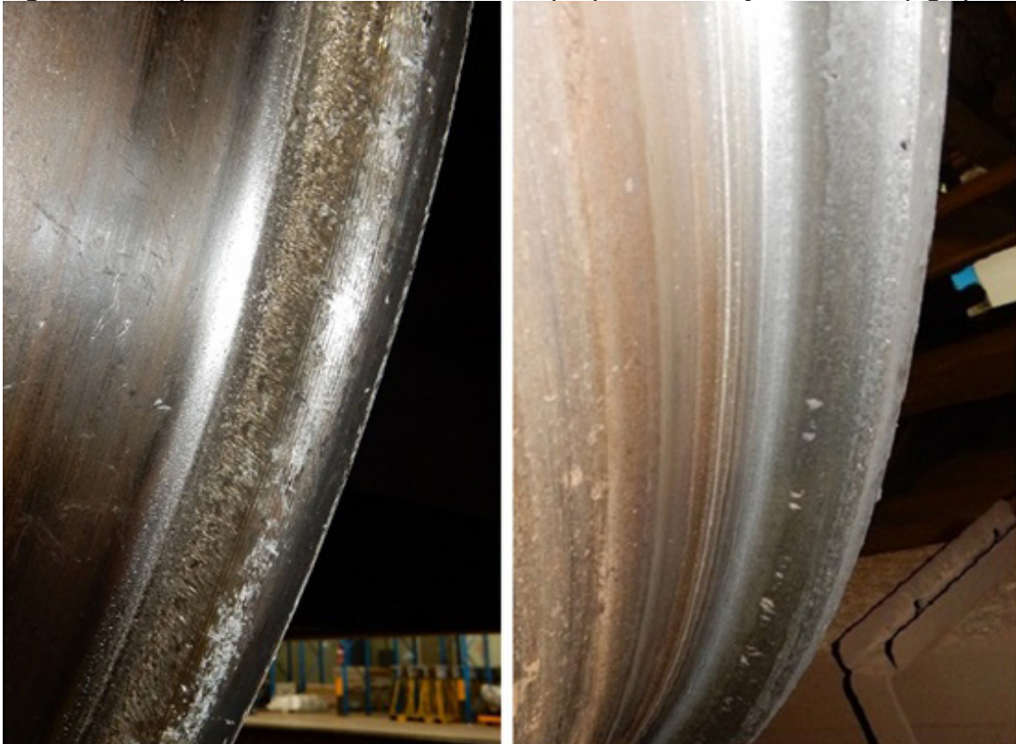
Figure 16: Comparison between derailed wheel (left) and normally worn wheel (right)
