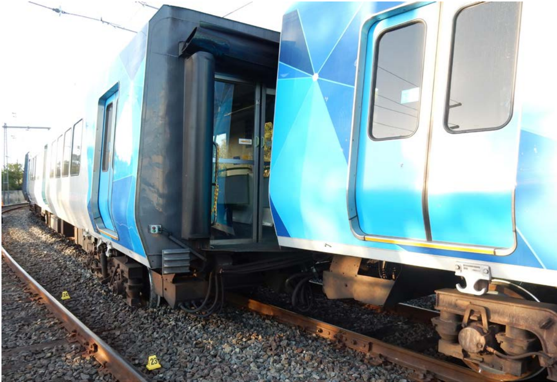
Figure 2: View of the derailed leading-end bogie of the second car
